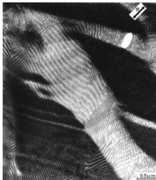
Figure 10. TEM micrograph of craze structure in a PS- b -PBMA diblock copolymer with hexagonal packed PBMA cylinders (SBM76, \Phi_{PS} = 0.76 , M_n = 459 kg/mol); stained with \text{RuO}_4 .
